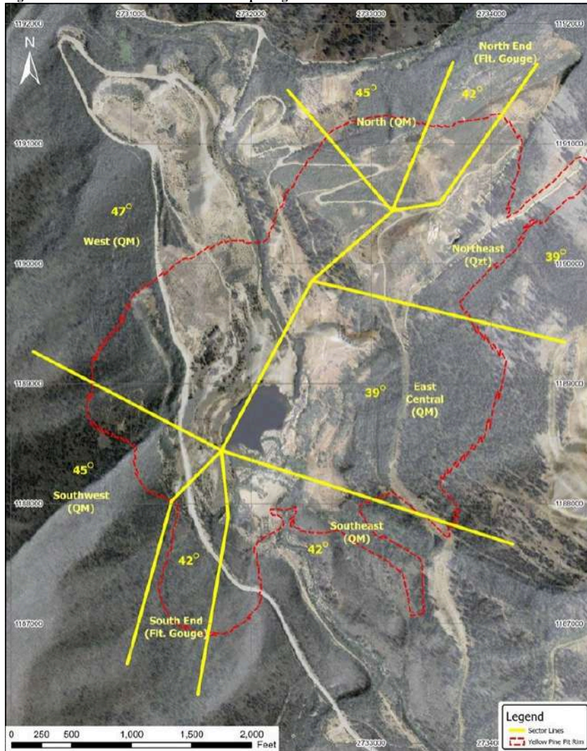
Figure 12-2: Yellow Pine Overall Pit Slope Angles
