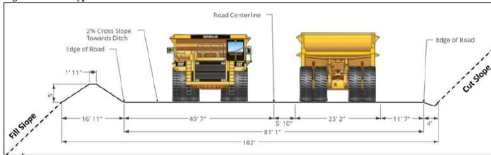
Figure 12-12: Typical Haul Road Cross-Section
