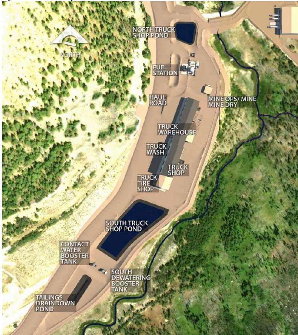
Figure 15-4: Truck Shop Area Detail
